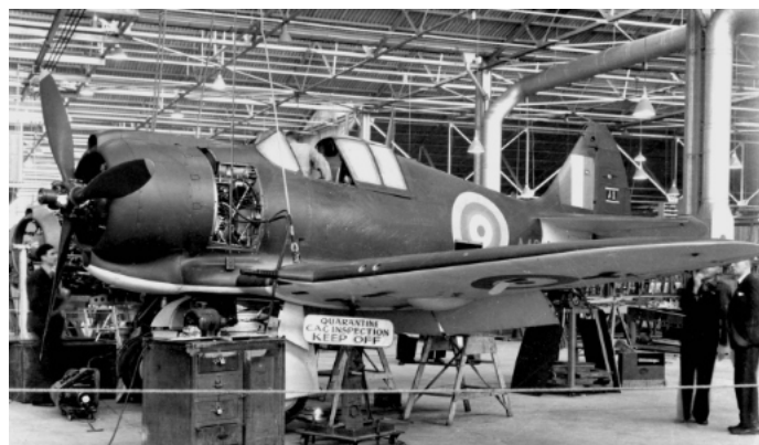
Above: The first Boomerang nears completion at CAC. Note the batch number A1 taped to the rudder. The nose of the aircraft is suspended above the floor and an external hydraulic pump is attached, most likely for undercarriage retraction tests. Official RAAF fuselage cockades at this time included a yellow outer band.
