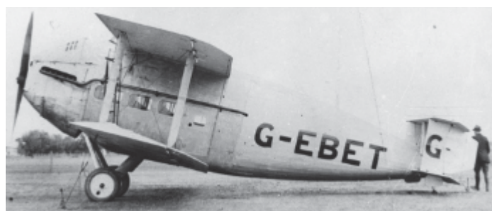
Above: The Vickers Vulcan tied down at an unknown location. The streamlined but very deep elliptical-section fuselage is obvious. Photo: NLA
