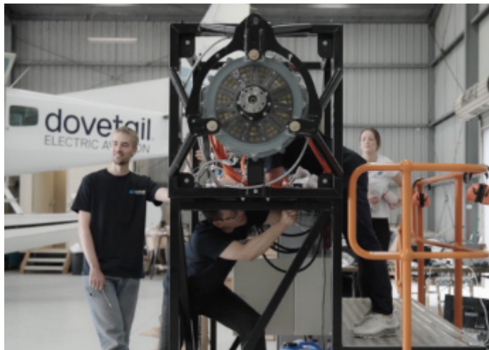
Above: A magniX electric motor mounted on Dovetail's ground test-rig. Photo: Dovetail Electric Aviation.
