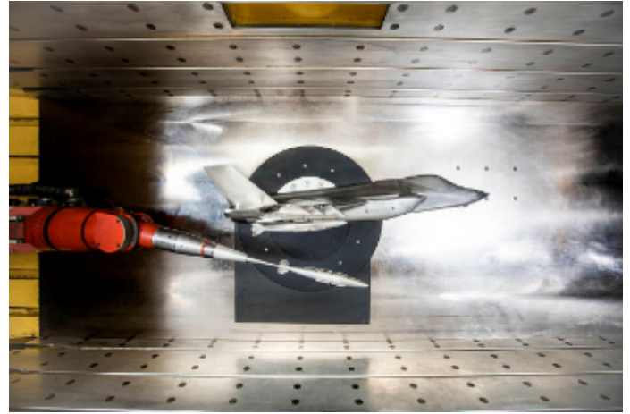
Above: Another view of the model of the F-35A mounted on the sidewall of the Defence Science and Technology Group Transonic Wind Tunnel with model of the GBU-31 (V1) weapon during pre-test grid check (Department of Defence).
