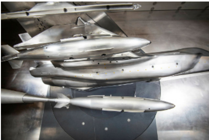
Above: Model of the F-35A mounted on the sidewall of the Defence Science and Technology Group Transonic Wind Tunnel with model of the GBU-31 (V1) weapon during pre-test grid check (Department of Defence).
