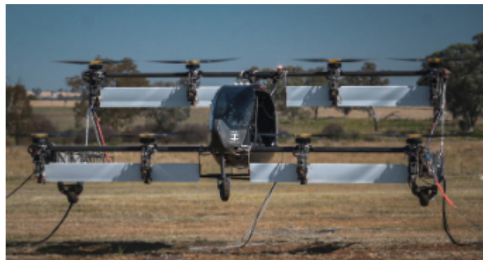
Above: The Vertiiia eVTOL aircraft hovering at low altitude during its first tethered test flight (AMSL Aero).
